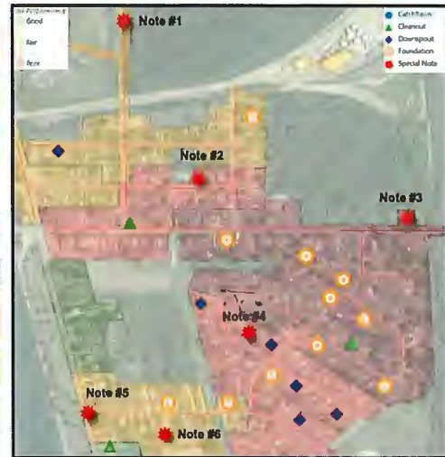
Figure 4: Smoke Testing Observations - North Central
