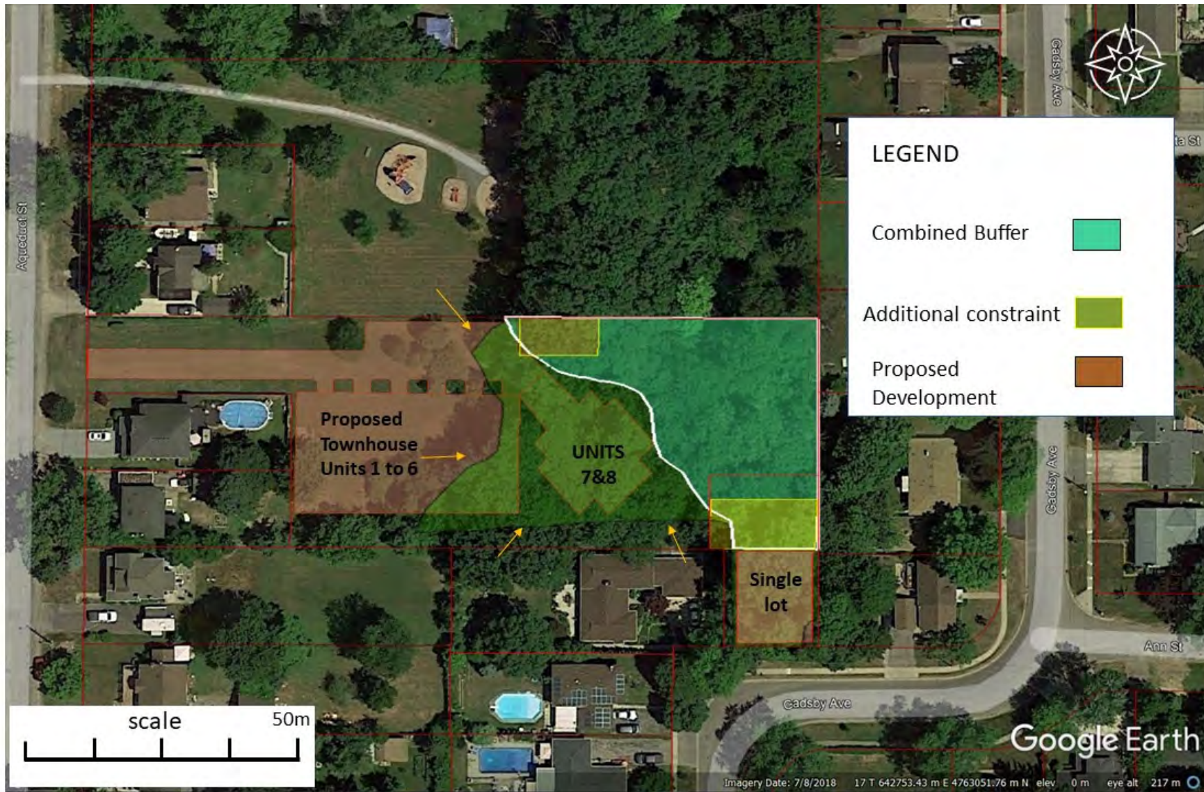
Figure 24. Proposed development area overlaid onto the most recent publicly available aerial imagery of the subject lands with combined buffer and additional constraints added to protect ecological functions confirmed within the remaining woodland with Aqueduct Park and the Subject lands. Arrows are pointing to the woodland boundary. Imagery courtesy of Google Earth July 2018.
